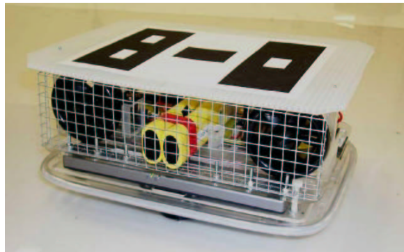
Figure 2: An MVWT vehicle rests on three ball casters and supports a stripped down laptop, batteries and two ducted fans for propulsion.
