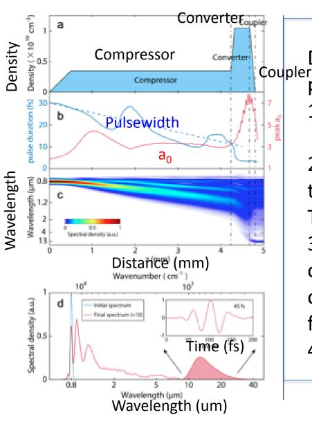
Different regions of the structure perform different functions Compressor compresses the pulse 1) from 30-10 fs by SPM/GVD 2) Converter rapidly down converts the pulse while further compressing it. The a0 of the pulse rapidly increases 3) The longest wavelength components slip back by GVD into the cavity where they are phase locked to form a near transform limited pulse 4) The pulse width is 1-2 cycles
