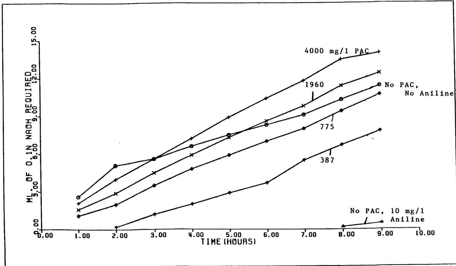
Figure 32: Initial Carbon Dose Experiment: Caustic Uptake vs Time
