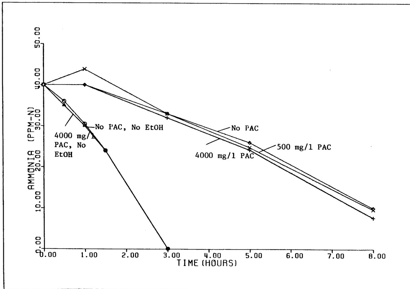
Figure 44:  $\text{NH}_3$  vs Time for Variable Carbon Dose (Ethanol, 2500 mg/l)
