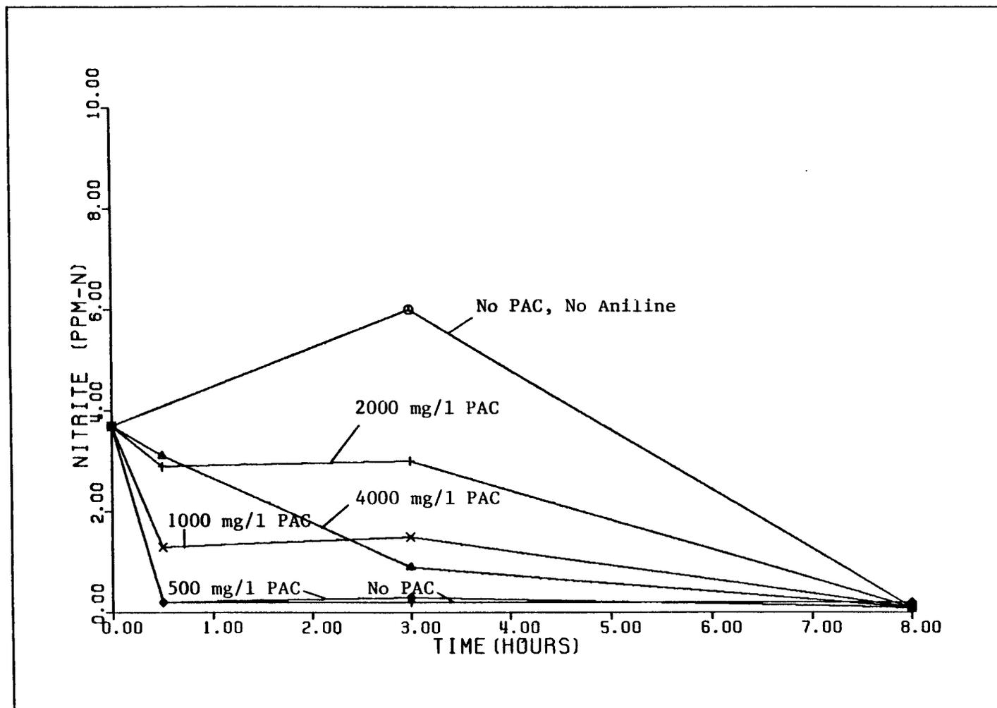
Figure 48:  $\text{NO}_2$  vs Time for Variable Carbon Dose (10 mg/l Aniline)
