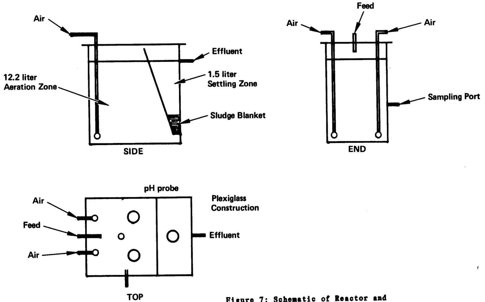
Figure 7: Schematic of Reactor and Associated Apparatus
