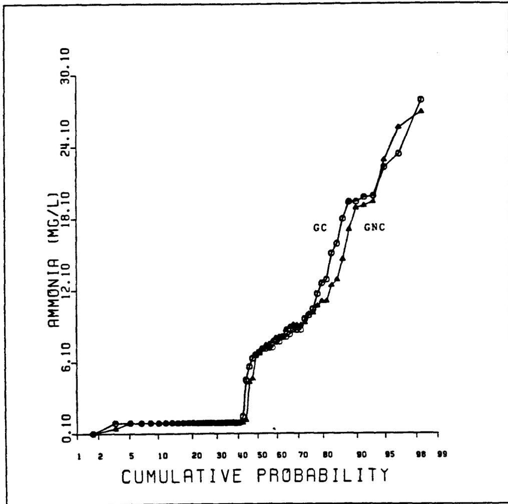
Figure 59: Cumulative Effluent Ammonia Probability for Glucose Reactors
