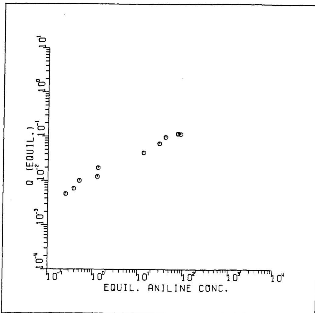
Figure 19: Aniline Isotherm:  $\log q_e$  vs.  $\log C_e$  for Carbon
