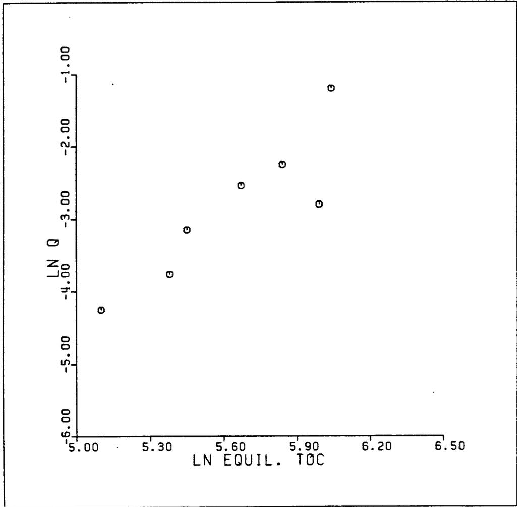
Figure 10: Refinery Wastewater Isotherm:  $\ln q_e$  vs  $\ln C_e$  for PAC
