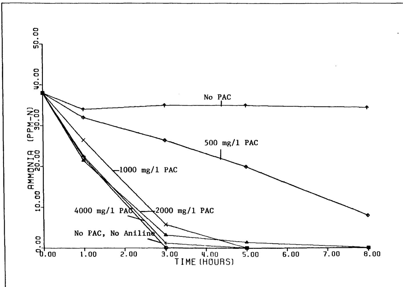
Figure 36:  $\text{NH}_3$  vs Time for Variable Carbon Dose (10 mg/l Aniline)
