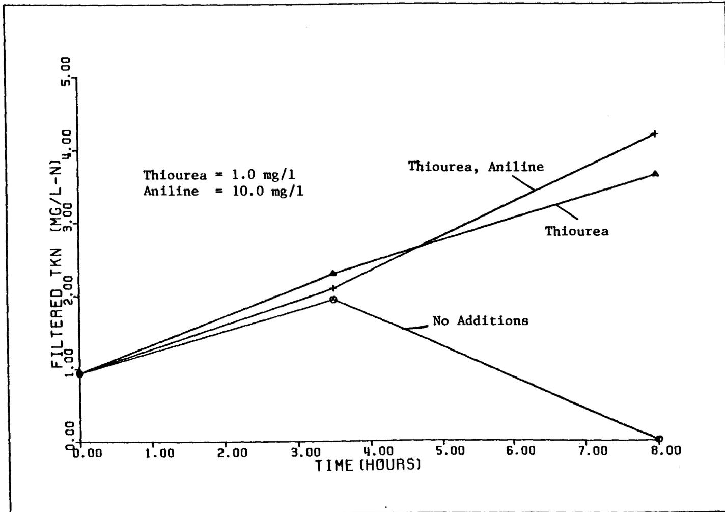
Figure 34: Filtered TKN with Time
