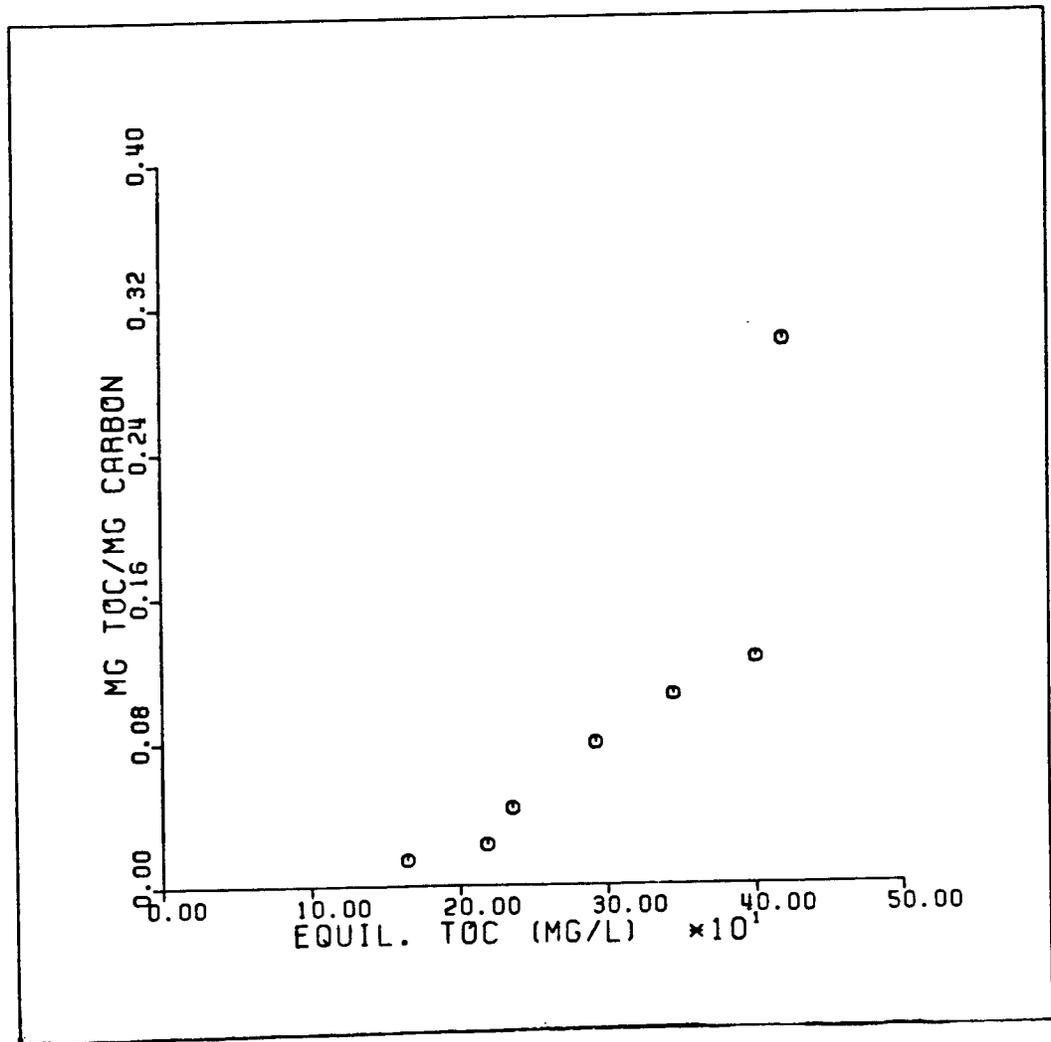
Figure 9: Refinery Wastewater Isotherm:  $q_0$  vs  $C_0$  for PAC
