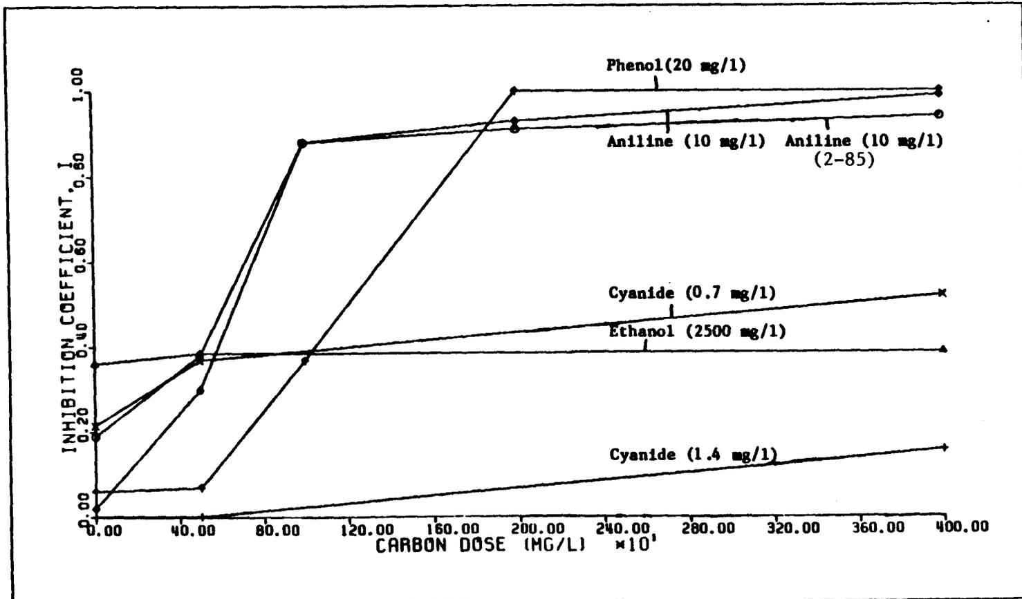
Figure 57: Inhibition Coefficient,  $I$  ( $\text{NH}_3$ ) vs PAC Dosage
