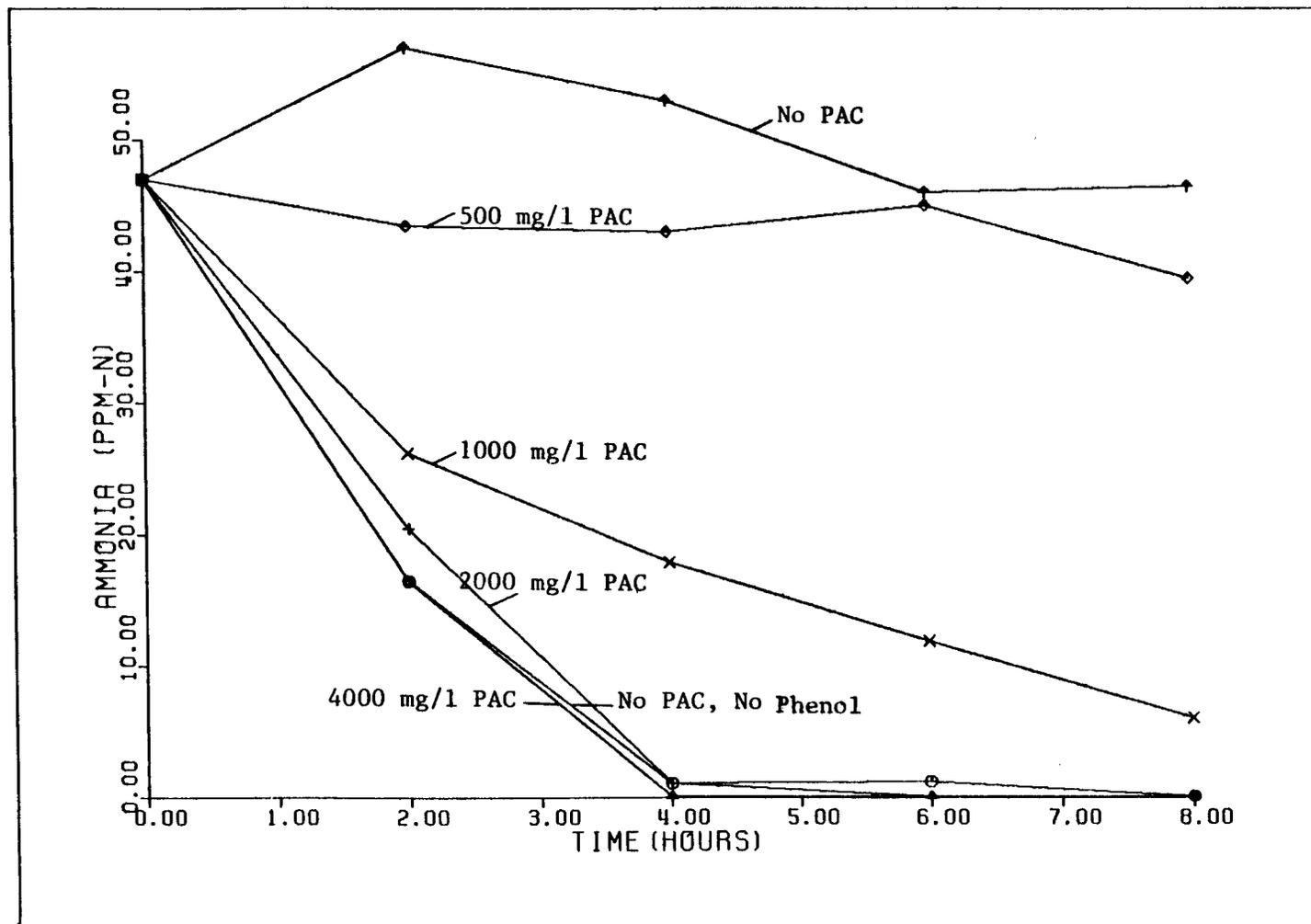
Figure 38:  $\text{NH}_3$  vs Time for Variable Carbon Dose (20 mg/1 Phenol)
