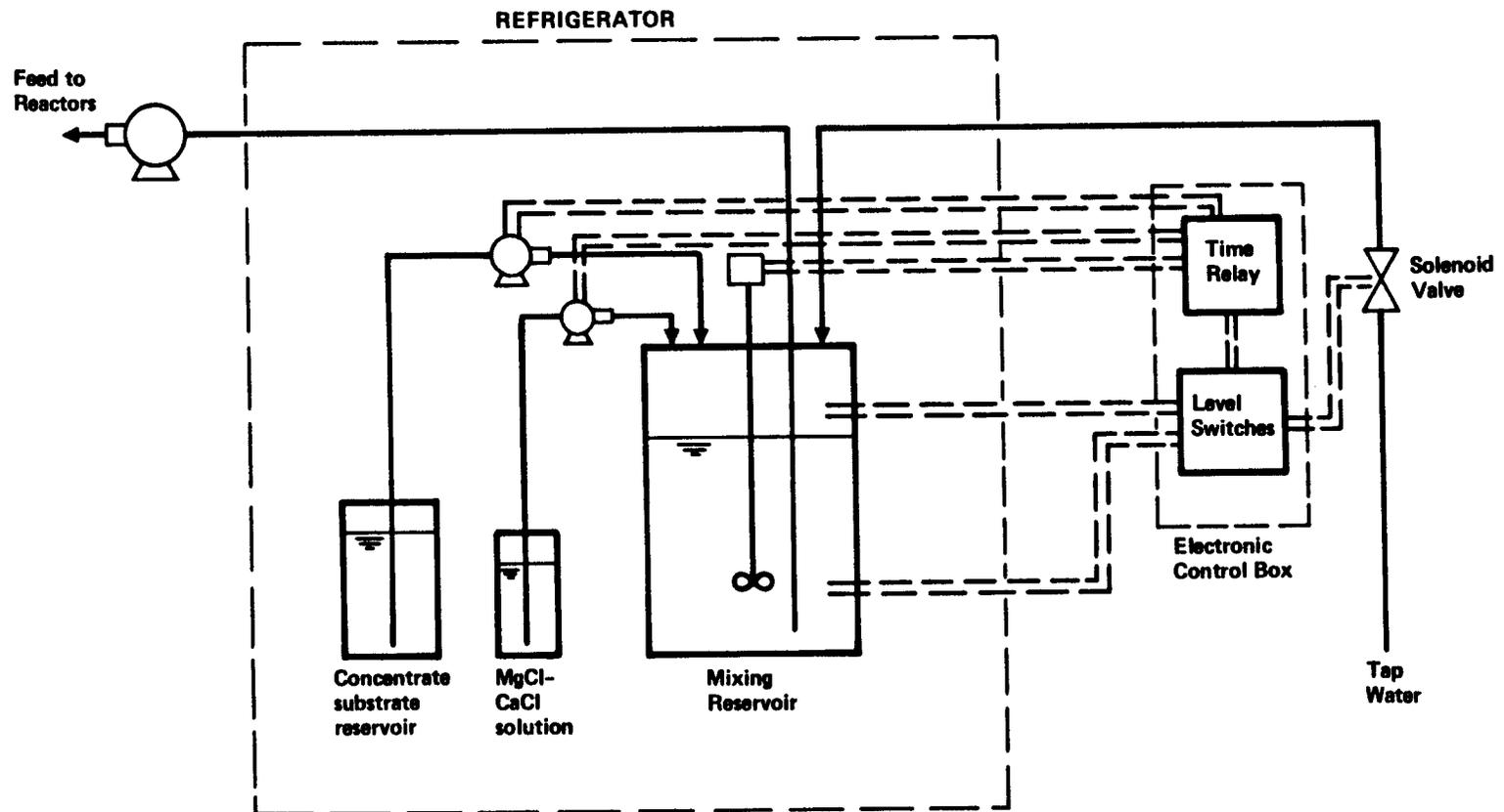
Figure 8: Schematic of Substrate Dilution System
