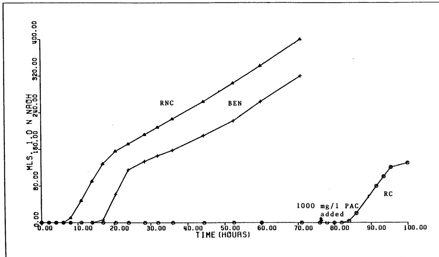
Figure 23: First Chronic Experiment: Caustic Uptake vs Time
