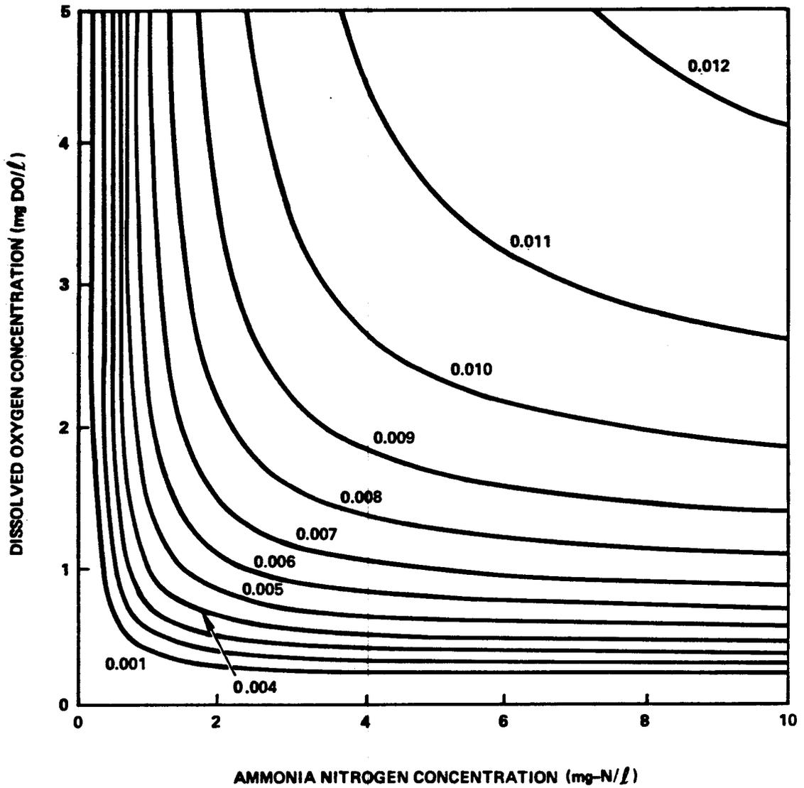
Figure 4: Net Growth Rate Contours Versus Ammonia Nitrogen and Dissolved Oxygen Concentration. (Numbers on curves indicate growth rate,  $\text{hrs}^{-1}$ . (After Stenstrom and Poduska, 1980).
