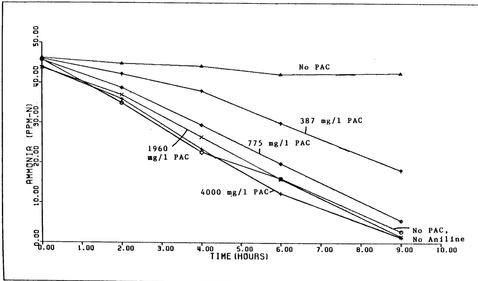
Figure 30: Initial Carbon Dose Experiment: Ammonia vs Time
