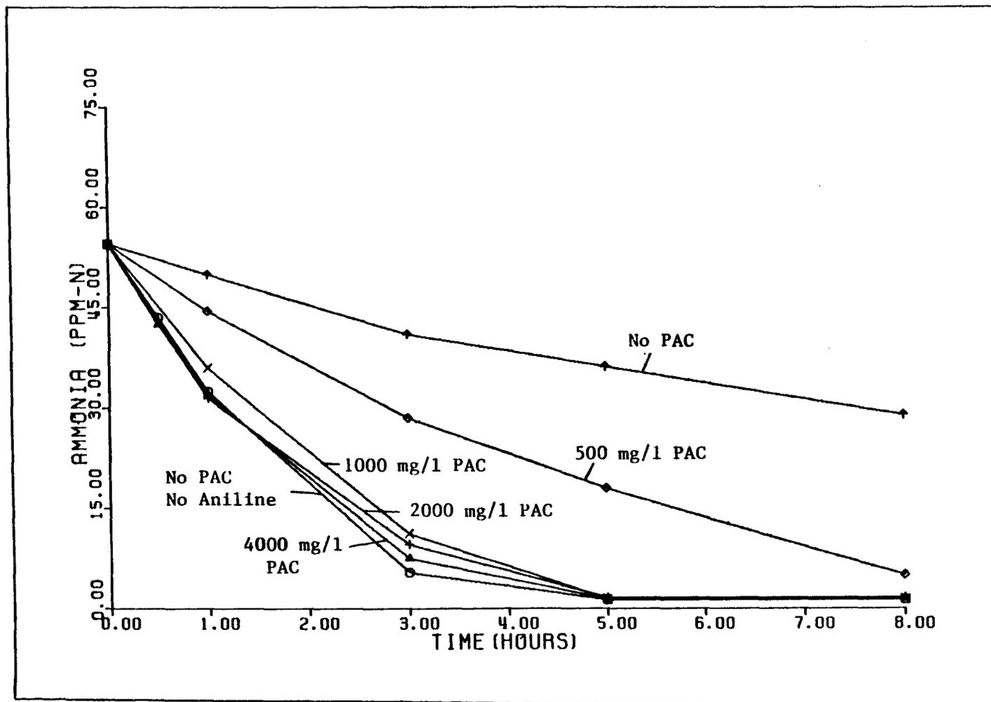
Figure 46:  $\text{NH}_3$  vs Time for Variable Carbon Dose (Aniline, 10 mg/l)
