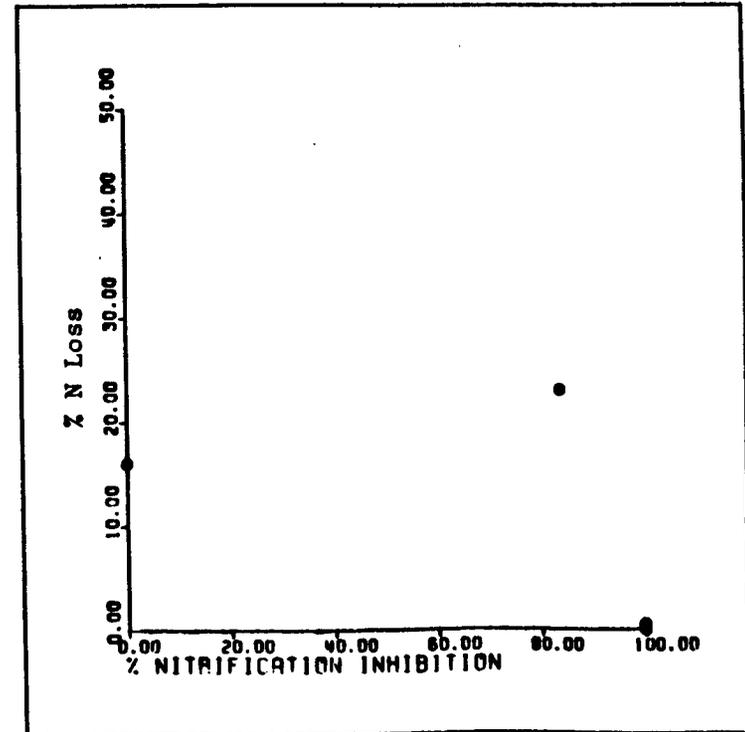
Figure 56: % Inhib. vs % N Loss (Cyanide, 1.4 mg/l)
