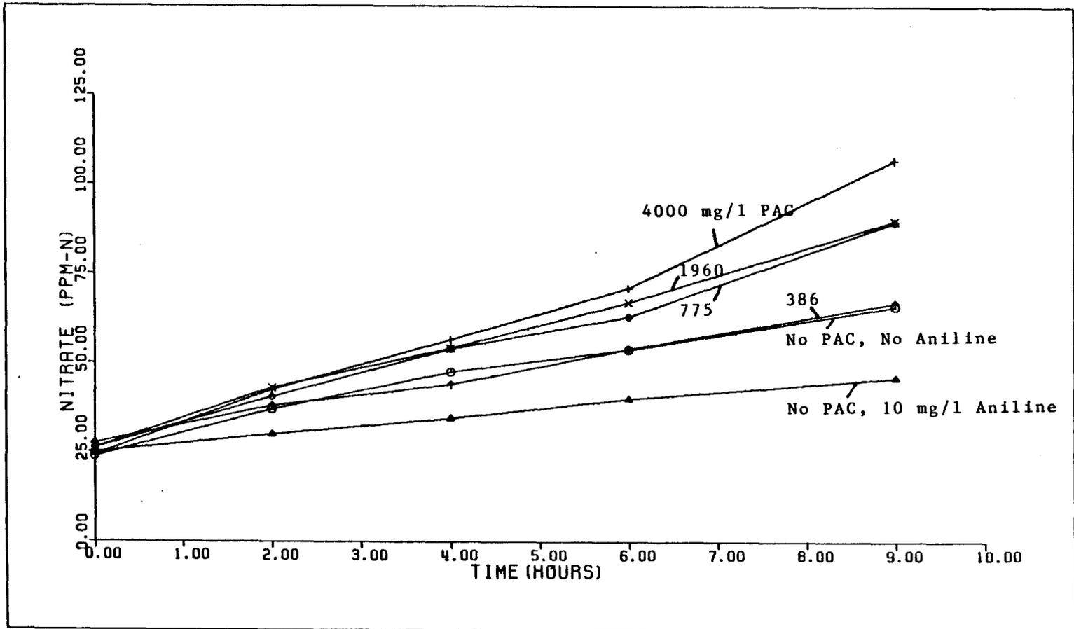
Figure 31: Initial Carbon Dose Experiment: Nitrate vs Time
