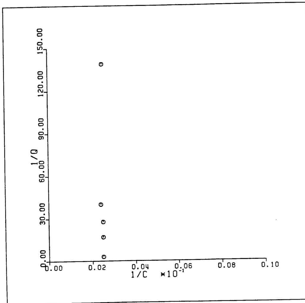
Figure 14: Refinery Wastewater Isotherm:  $1/q$  vs  $1/C$  for Bentonite
