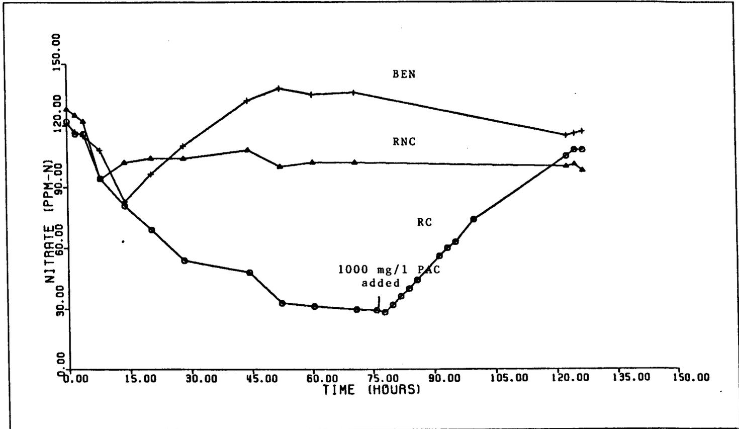
Figure 24: First Chronic Experiment: Nitrate vs Time
