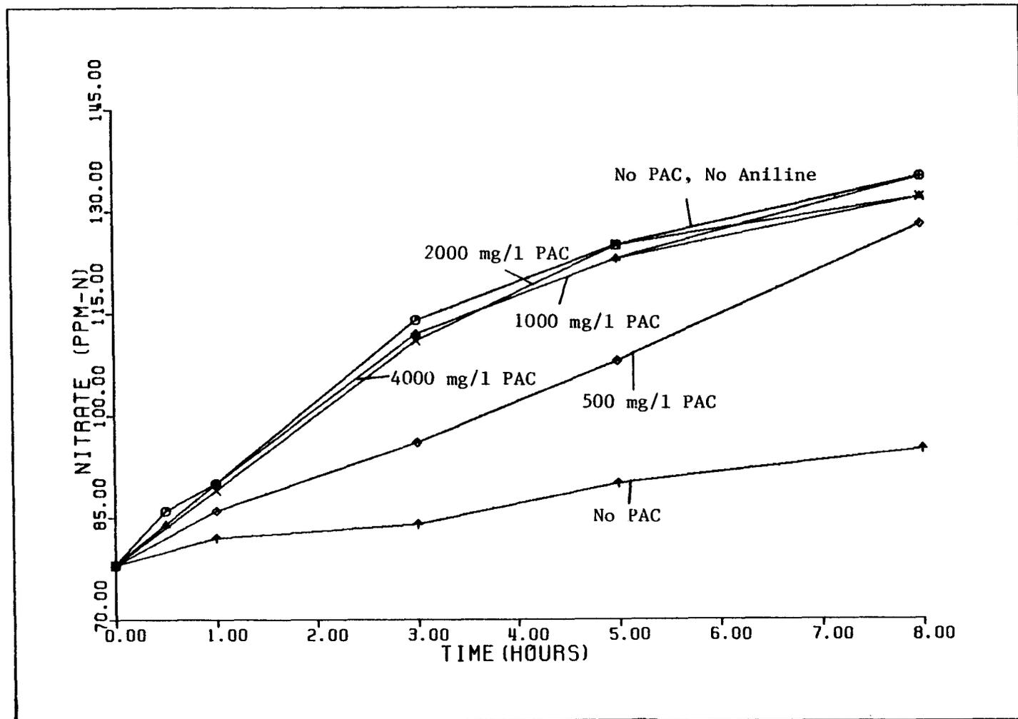
Figure 47:  $\text{NO}_3$  vs Time for Variable Carbon Dose (10 mg/l Aniline)
