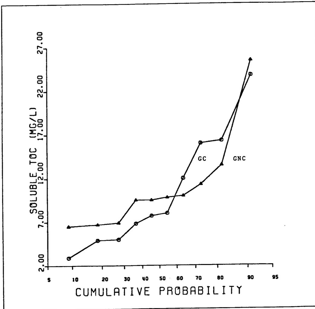
Figure 17: Cumulative SOC Probability For Glucose Reactors
