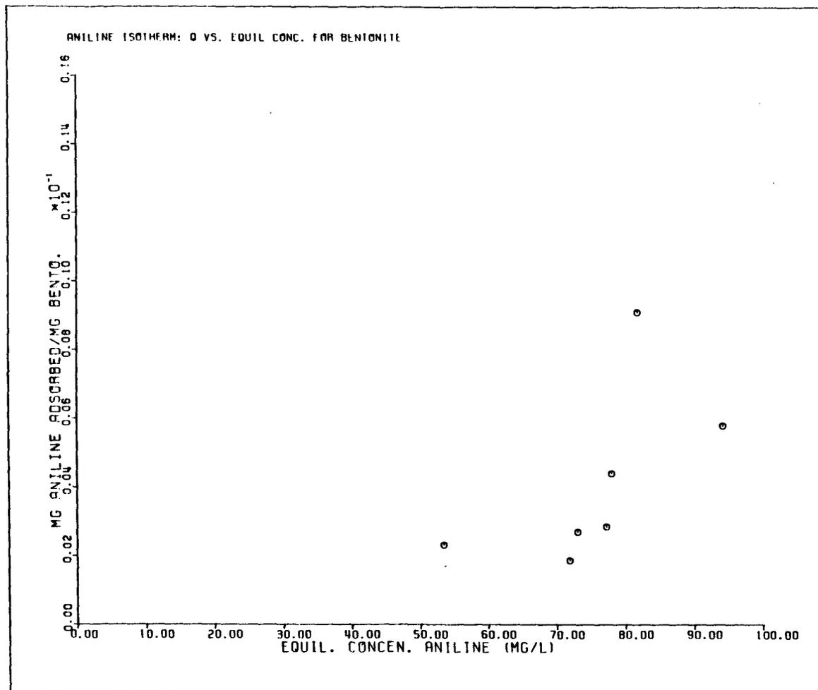
Figure 20: Aniline Isotherm:  $q_0$  vs  $C_0$  for Bentonite
