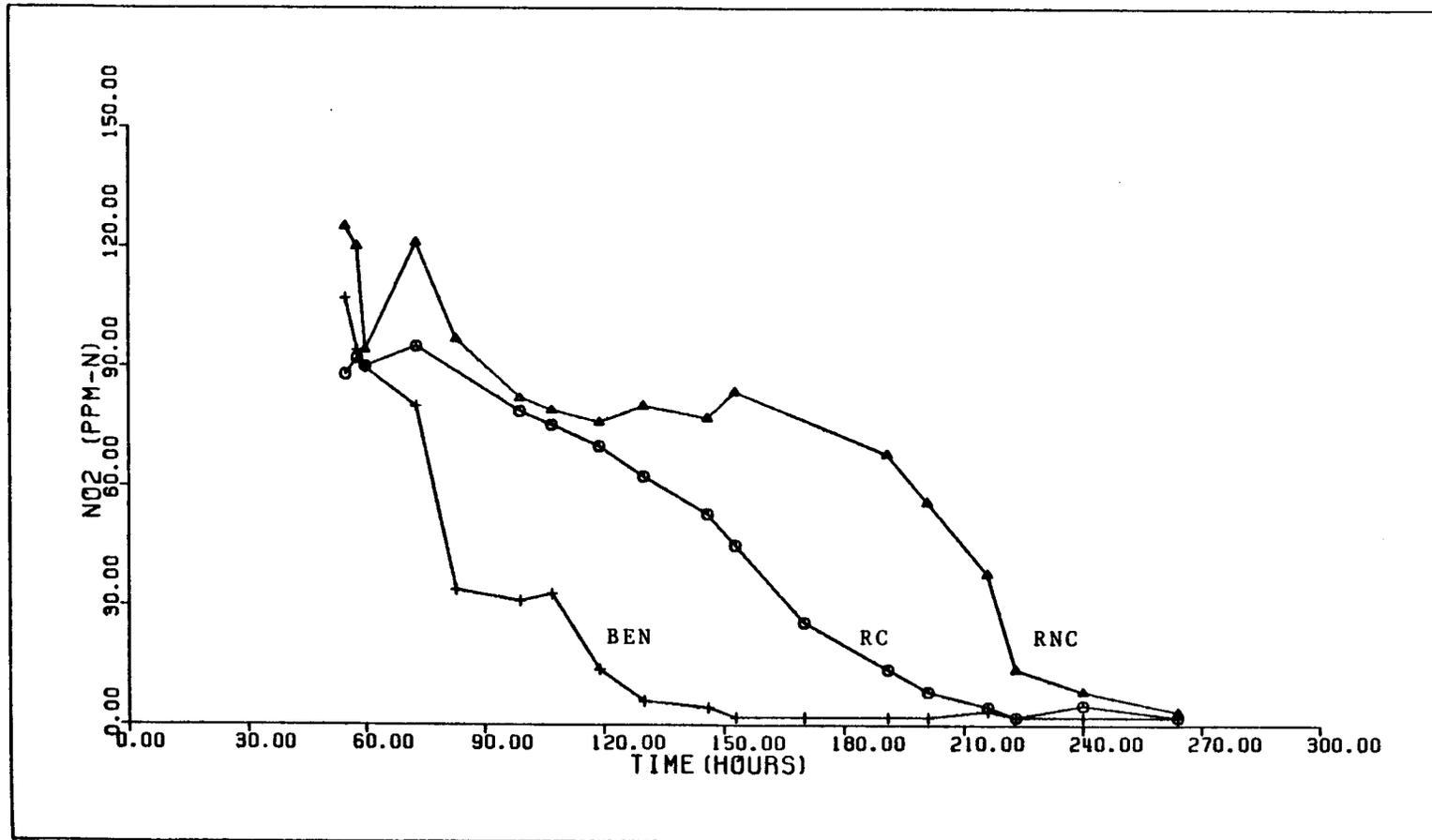
Figure 29: Second Chronic Experiment: Nitrite vs Time
