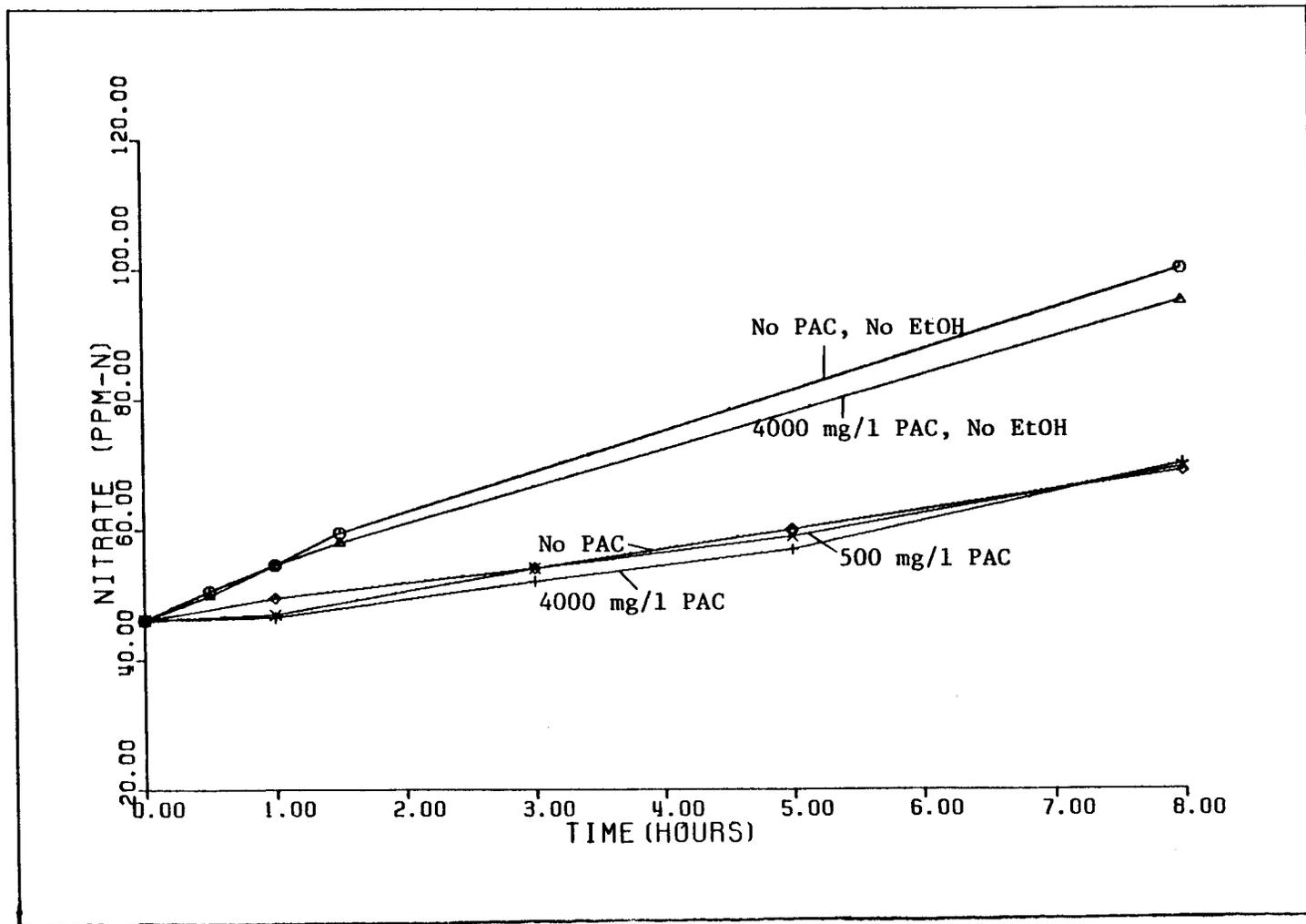
Figure 45:  $\text{NO}_3$  vs Time for Variable Carbon Dose (Ethanol, 2500 mg/l)
