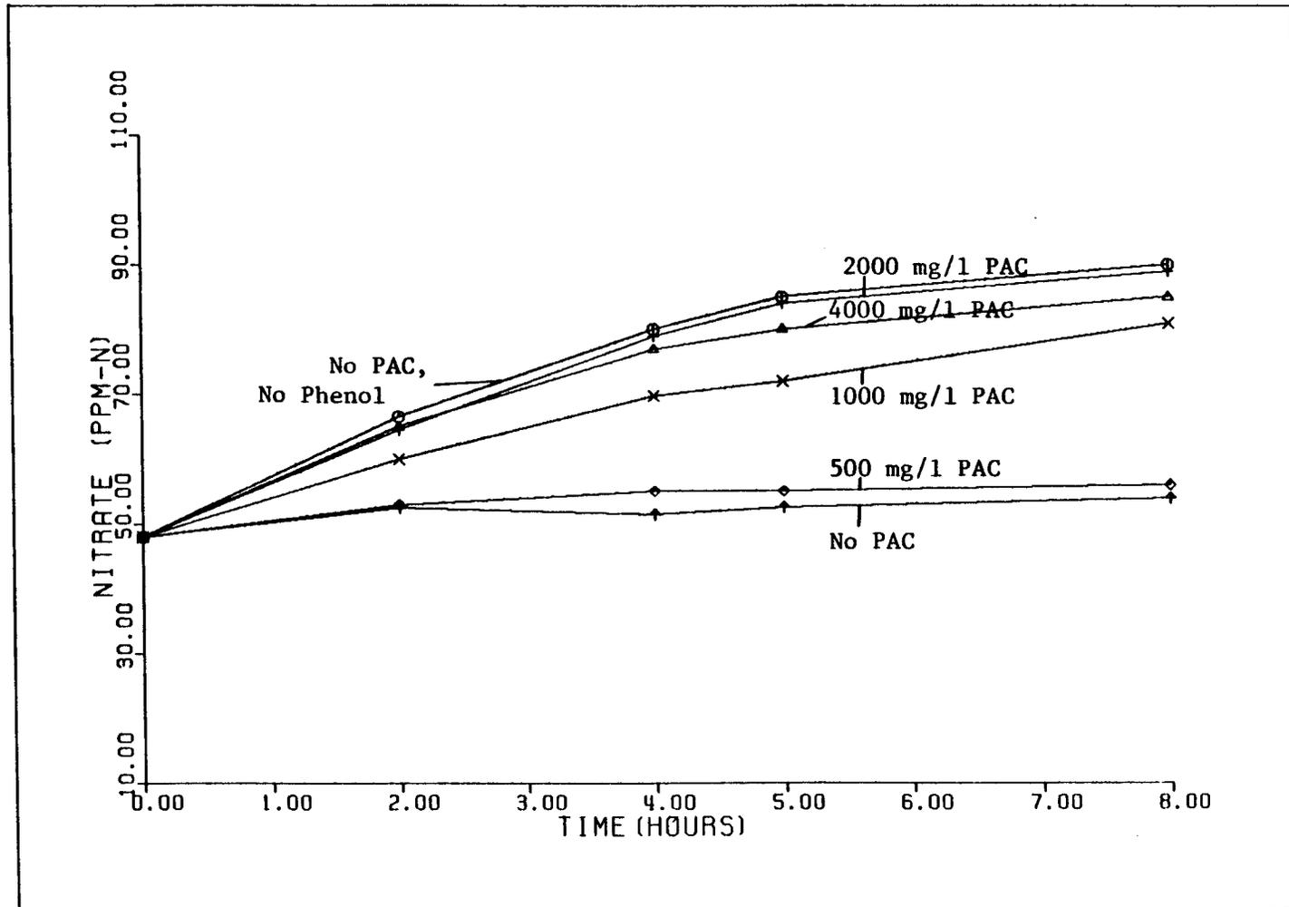
Figure 39:  $\text{NO}_3$  vs Time for Variable Carbon Dose (20 mg/l Phenol)
