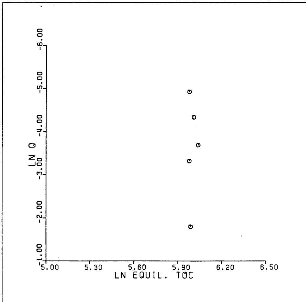
Figure 13: Refinery Wastewater Isotherm:  $\ln q_e$  vs  $\ln C_e$  for Bentonite
