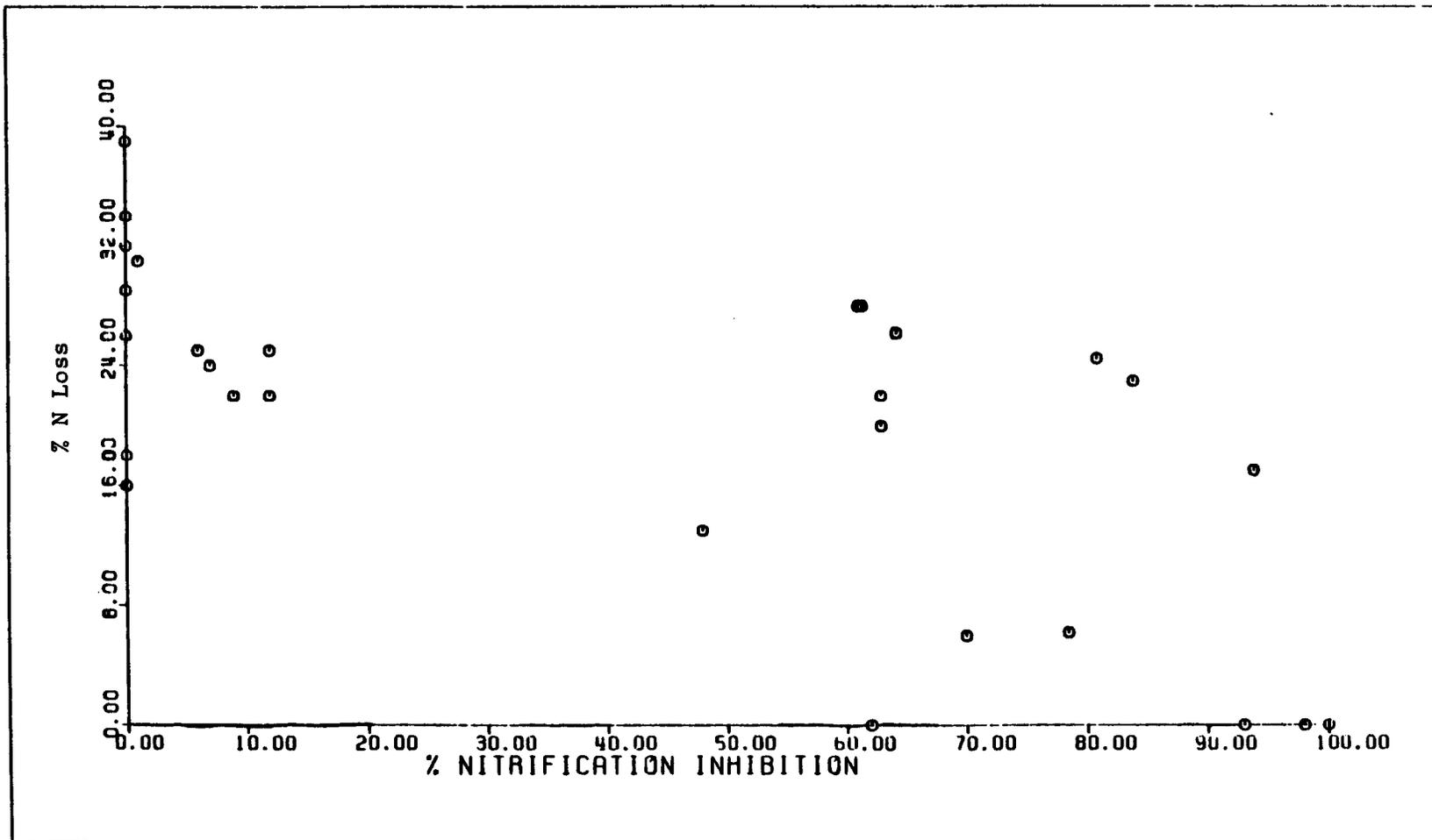
Figure 50: % Inhibition vs % N Loss for All Carbon Dose Experiments
