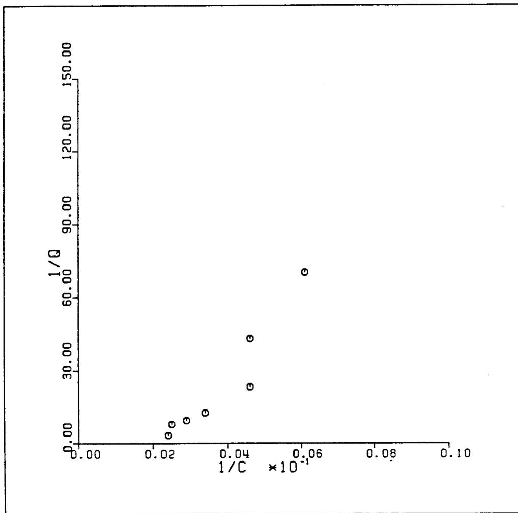
Figure 11: Refinery Wastewater Isotherm:  $1/q$  vs  $1/C$  for PAC
