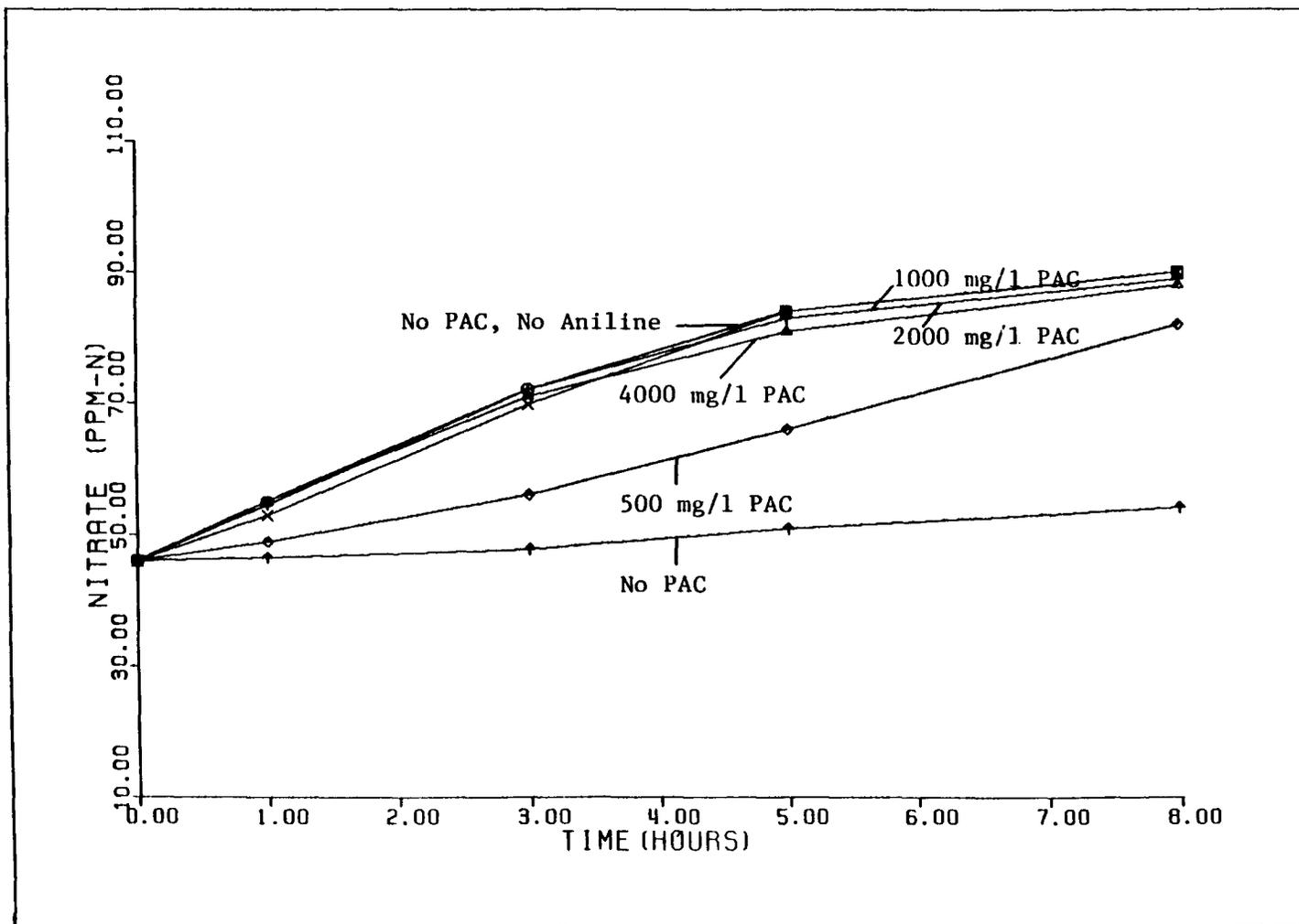
Figure 37:  $\text{NO}_3$  vs Time for Variable Carbon Dose (10 mg/l Aniline)
