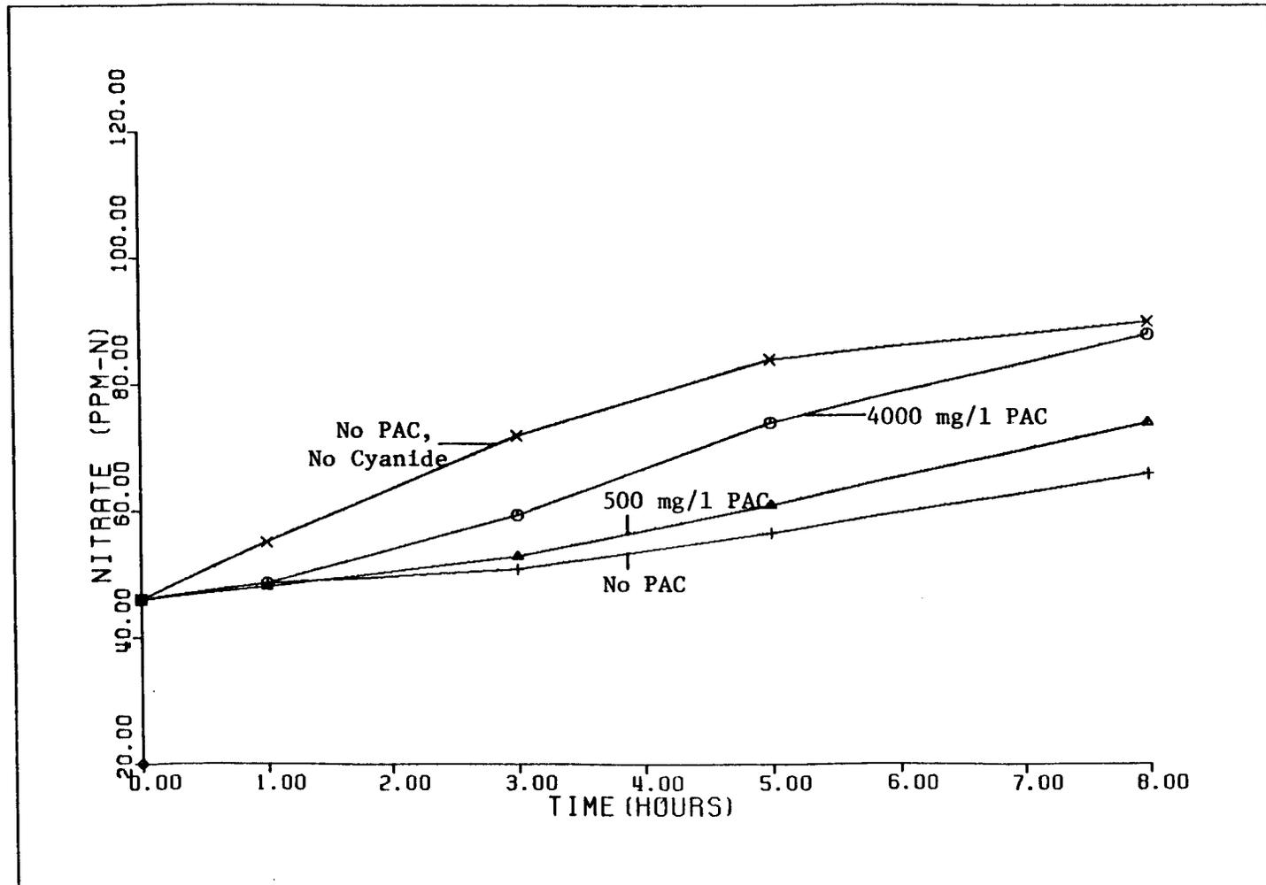
Figure 41:  $\text{NO}_3$  vs Time for Variable Carbon Dose (0.7 mg/1 Cyanide)
