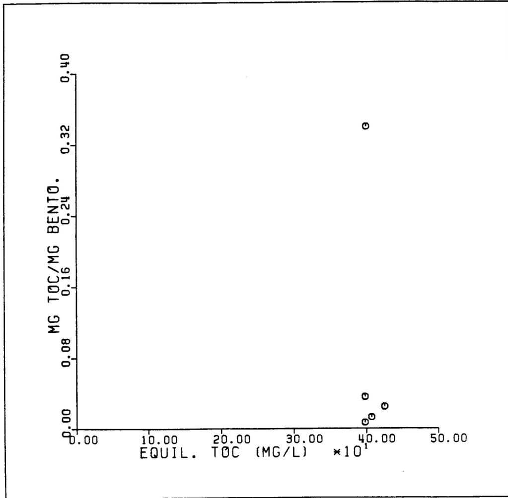
Figure 12: Refinery Wastewater Isotherm:  $q_e$  vs  $C_e$  for Bentonite
