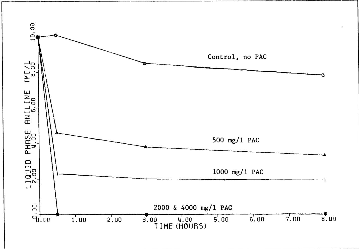
Figure 49: Liquid Phase Aniline Concentration vs. Time
