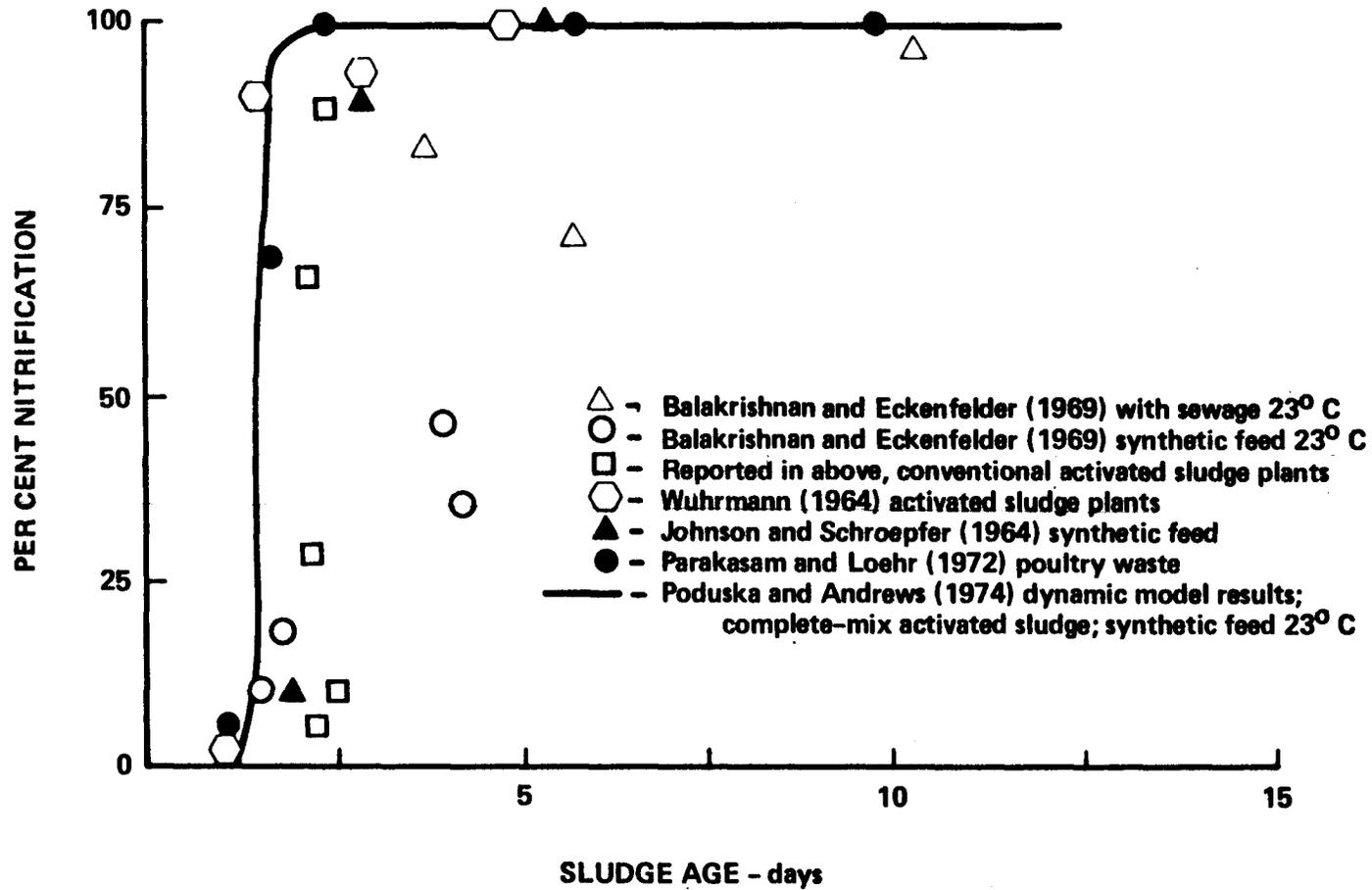
Figure 3: Comparison of Nitrification Data taken from the Literature and Results Predicted by the Steady State Model of Poduska and Andrews (After Poduska and Andrews, 1974)
