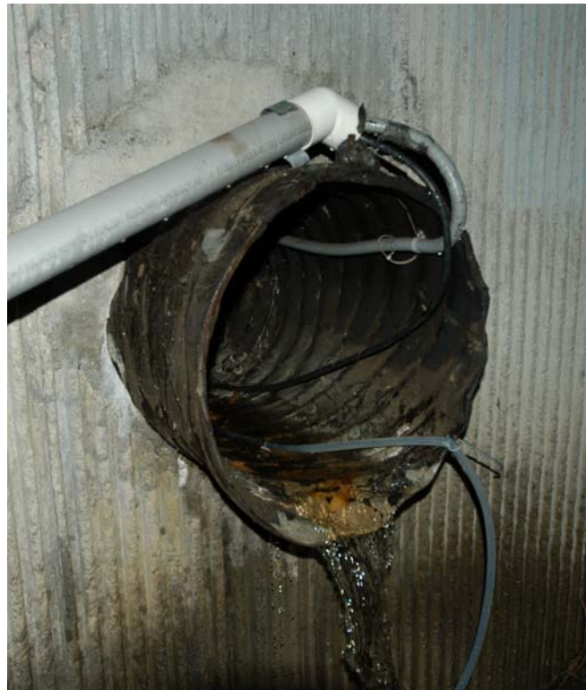
Figure 2.2 Pictures of Site 1, clockwise from the top: 1) site from a distance of 30 meters; 2) drainage pipe showing free waterfall and cables for level and velocity sensors, and 3) rain gage above the sound wall.
