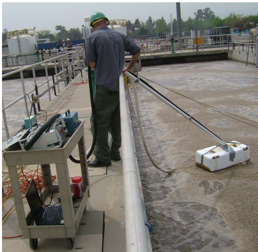
Figure 19. Real-time off-gas test with field prototype no. 2 and a small hood
