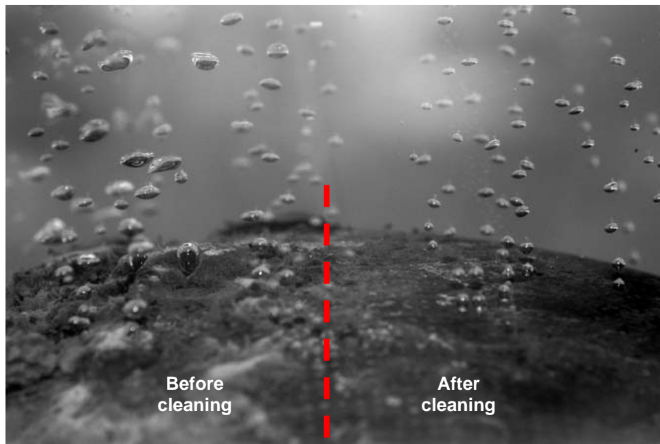
Figure 6. Photograph of a half-cleaned diffuser: before cleaned (left part of the diffuser) the diffuser was covered by a layer of biomass and the bubbles produced are big; after cleaned (right) the bubbles turn to smaller, similar to a new diffuser.
