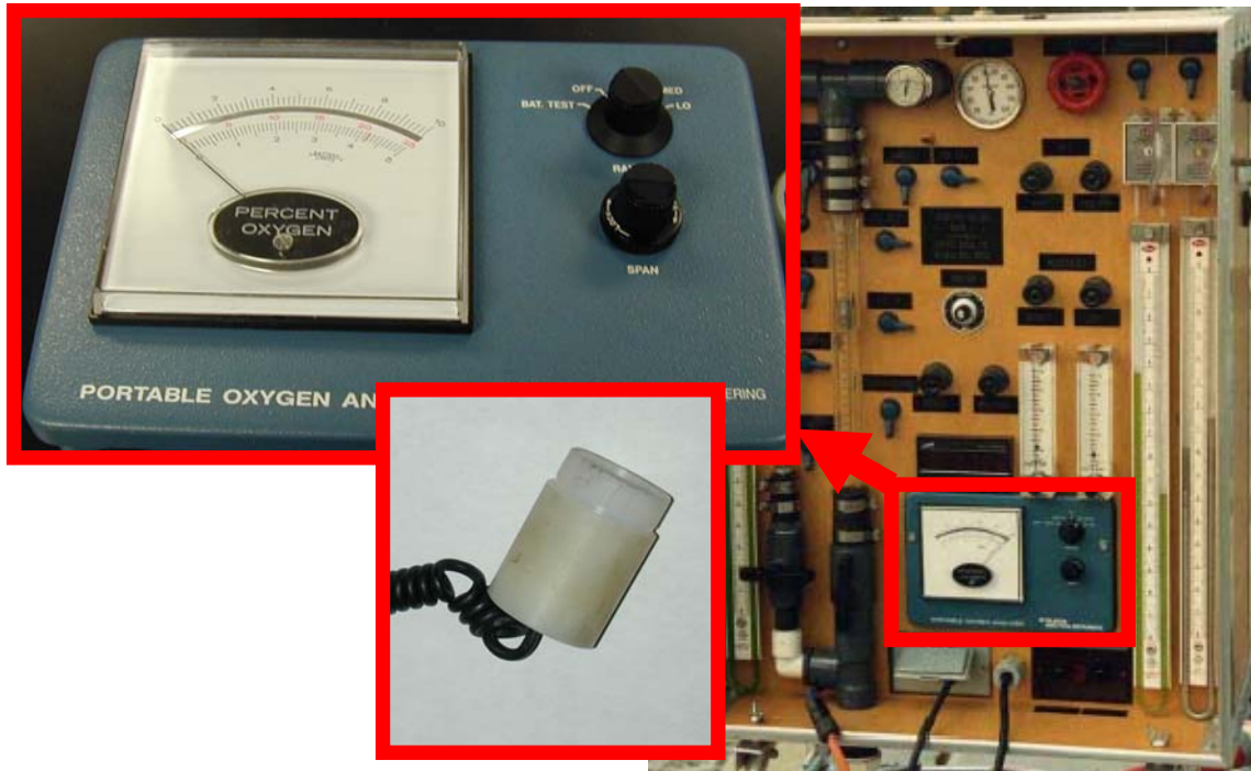
Figure A-5. Manual off-gas testing apparatus (Manufactured by Ewing Co.). Details show the oxygen purity meter and its fuel cell.
