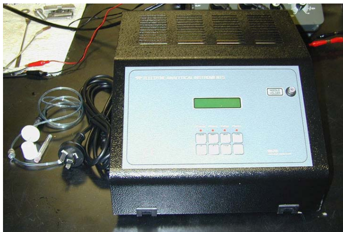
Figure 2. Lab-scale off-gas testing apparatus (Teledyne 9070 O 2 /CO 2 analyzer) used in our laboratory.
