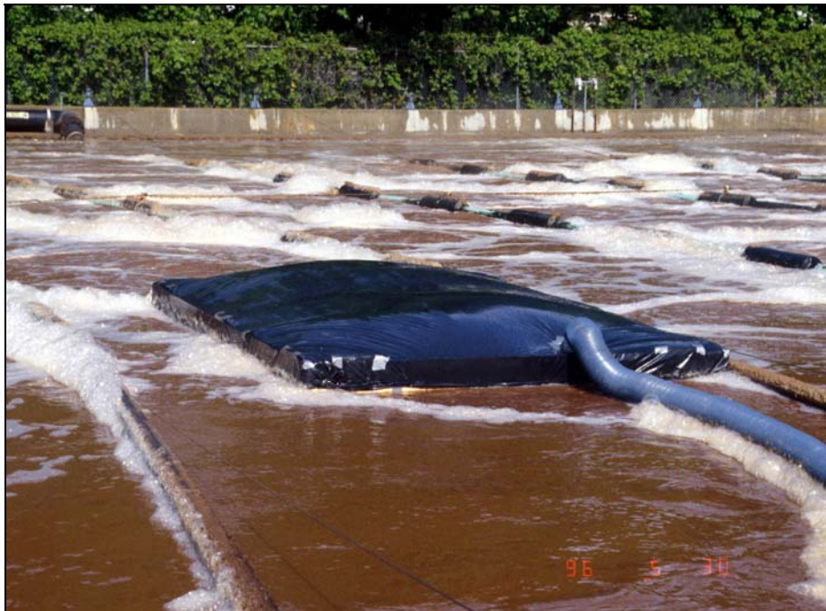
Figure. A-4 (a), (b) Off-gas capture hoods. 2x10', Styrofoam and aluminum frame (top); 5x8', wood and plastic sheets, built in situ (bottom).
