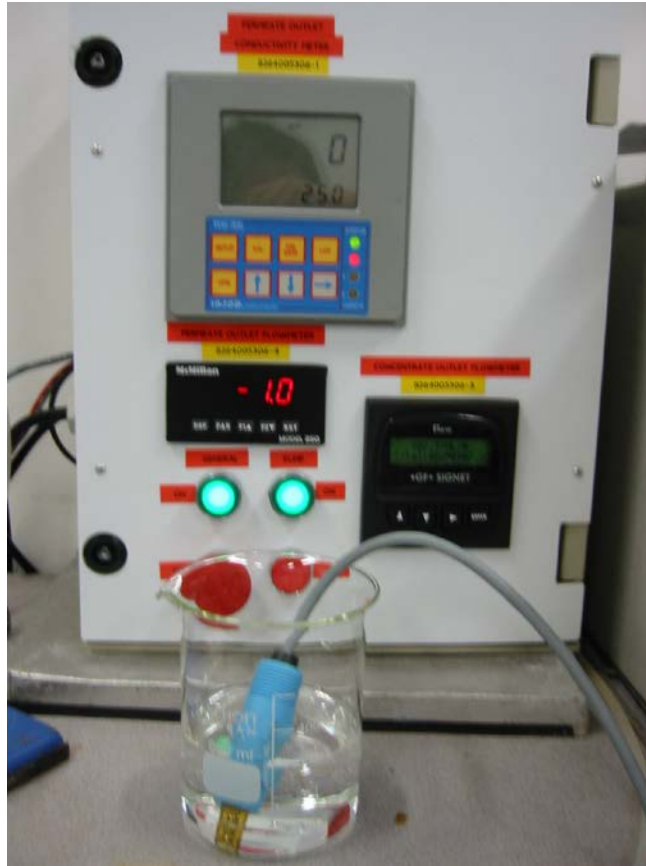
Figure 3.7: “On-line” conductivity meter used in the experiment.
