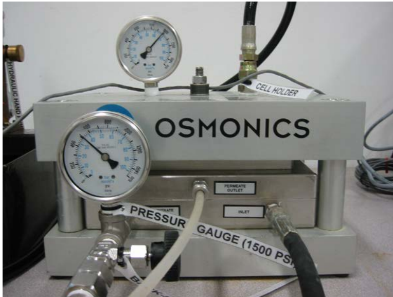
Figure 3.4: SEPA CF cell
