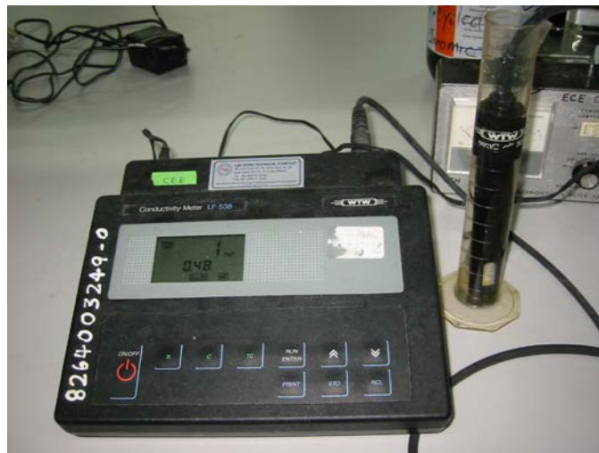
Figure 3.6: “Manual” conductivity meter used in the experiment
