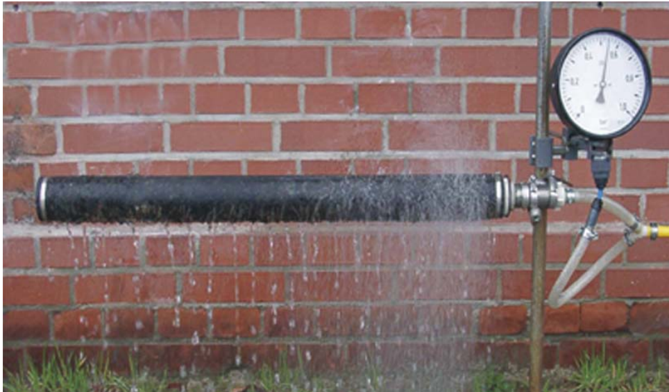
Figure 1--A fouled membrane diffusers is being tested. The fouling in the middle and left sections of the membrane diffuser are worse than the right section. The right section of the membrane diffuser produces more uniformed and smaller droplets.
