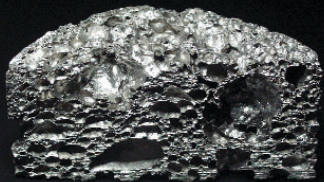
Sample of metal foams obtained by stirring low melting temperature alloys at high speed in a baffled beaker. The foam is stabilized by direct oxidation of the cell walls and no addition of oxide particles is required.
