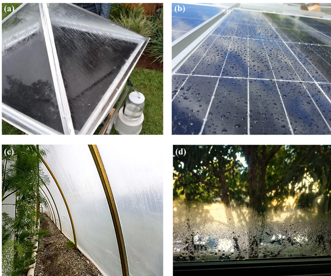
Fig. 1. Water droplets on the surface of (a) a solar still cover (photo by Michael J Scheepers, Design Engineer, Teq Design Central, mickeys@teq-dc.com), (b) a solar photovoltaic panel (credit: photograph reproduced with permission from GÜNAM, http://gunam.metu.edu.tr/ ), (c) a greenhouse cover (credit: photograph reproduced with permission from ZipGrow Incorporated, www.ZipGrow.com ), and of (d) a window.
